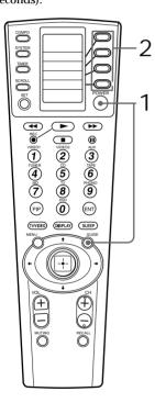
1 While pressing the POWER button, press the GUIDE button.
